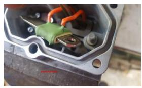
Apply pressure to the bottom of the plug, careful not to damage the wires or the resistor, and locate the 'C' clip onto the plug on the outside.
