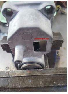
Fit the new 'O' ring over the electrical plug
