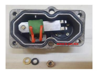
Set your multimeter to ohms and test the resistance of the bimetallic strip.
