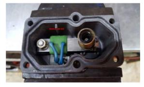
Now place the centre diaphragm section on the top body assembly. You must make sure that the springs sit into their seats in
