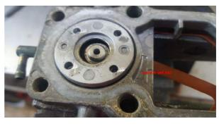
Lift off the spring mount to expose the small diaphragm.
