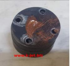
You have 4 Allen screws, put a small amount of grease on the thread, and tighten them firmly. Remember they are only small screws so don't go too hard and strip them.
