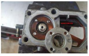
Turn the centre section housing over and remove the diaphragm assembly.
