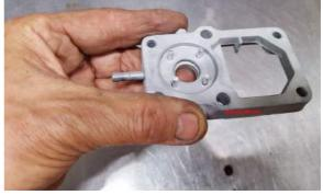
Place the diaphragm and centre pin over the rivets and again wipe the flat surface of the diaphragm with the gasket sealant
