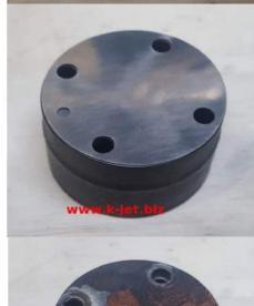
Put the cap on, just make sure there was no grease on the face of the cap otherwise it may affect how the shim operates.
