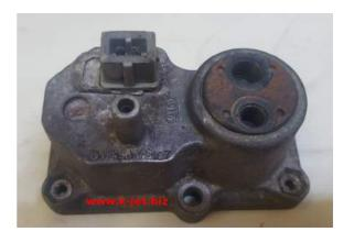
Undo the 6mm nut (size 10mm socket) so you can remove the bimetallic strip.
