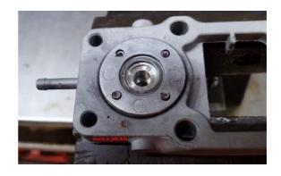
Flare the rivets over. Having the washers under the head of the rivets ensures that they don't move when you flare them over which could leave the diaphragm a bit loose. The rivets must be firm and the diaphragm seated tightly or else you will have vacuum leaks.
