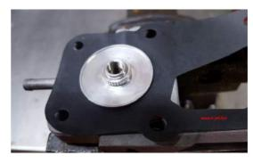
Now insert the centre adjustable screw. Note, often these don't have a 'O' ring seal on them, and in this picture I hadn't yet fitted it. Fit the 'O' ring and wipe a little bit of Vaseline on it before you screw it in. Screw it all the way in and then back it out about 3 turns.
