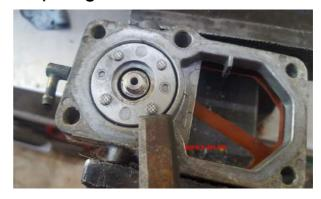
The rivet heads removed
