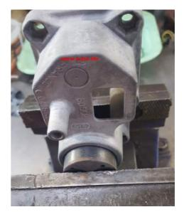
Put it in the vice as shown here and the tighten the vice until the fuel cell is sitting out about 4 to 5mm
