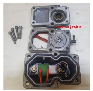
There are 2 springs, a 'hat' for the springs to sit on, and a pin which sits inside the hat and presses onto the fuel cell.
