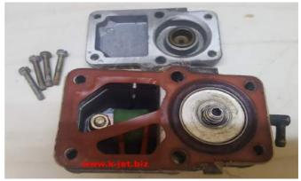
Remove the base and you will expose the diaphragm we will be replacing.
