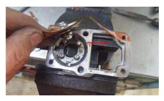
Remove the centre adjustable screw. You will reuse this screw in your new diaphragm.
