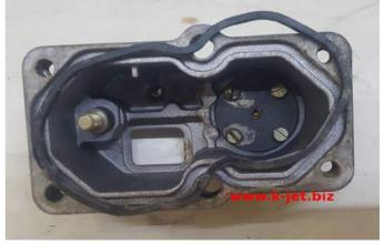
Only remove the fuel cell and the position of the bimetallic pin if you intend to reset the pressures.
